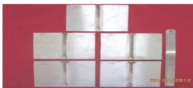
Fig 2(a).Photographs of Fabricated joints
