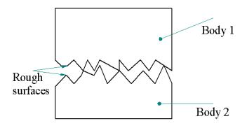
Fig.1 Two Surfaces in Contact
