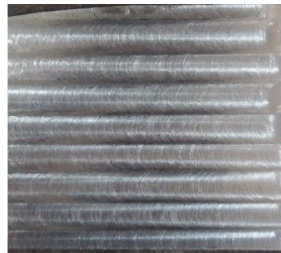
Fig. 9 Surface Finishing by the milling machine
