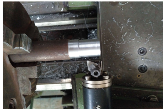
Fig. 2 Turning operation in Mild steel material for the measurement of cutting force
