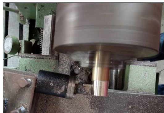
Fig. 3 Turning operation in Brass material for the measurement of cutting force
