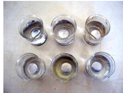
Fig. 1 Immersion corrosion test setup
