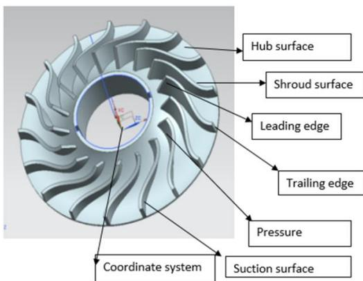
**Fig.3 Hub with integrated blades**
