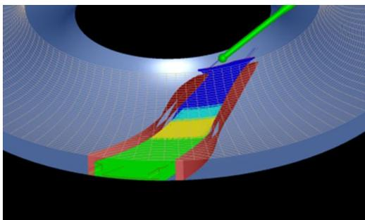
**Fig. 10 Generation of tool path Step for vanes**
