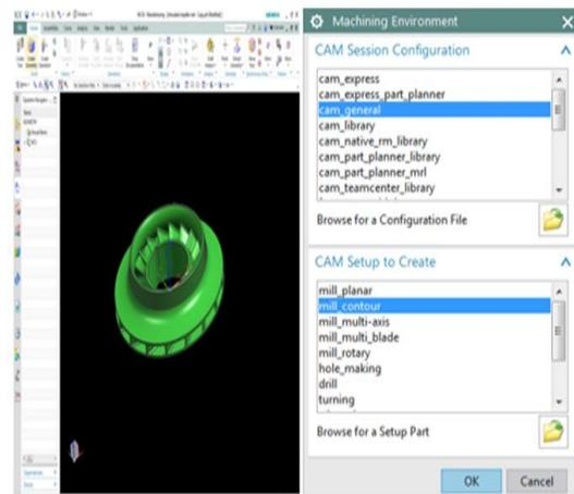
**Fig. 7 Frame that shows tool-path generation module**
