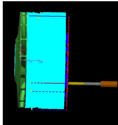
**Fig. 16** Tool path generation for finishing operation
