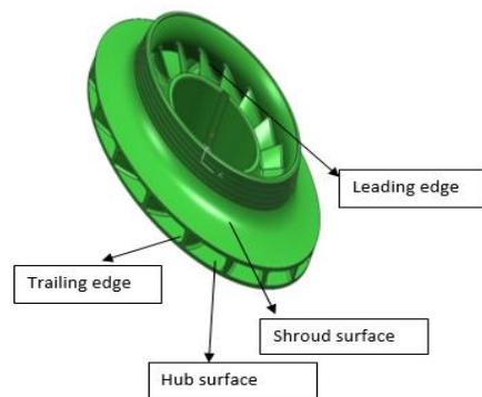
**Fig. 5 Complete assembly of 3D Shrouded Impeller**
