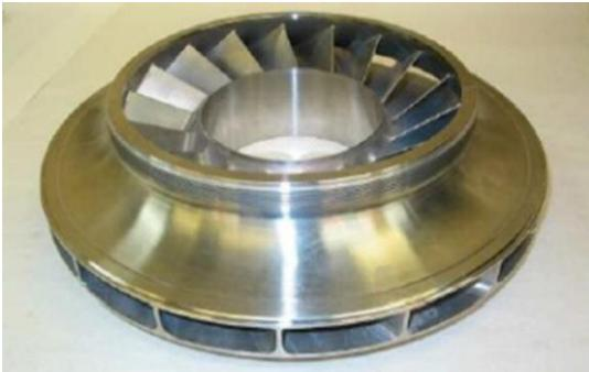
**Fig. 1 3D shrouded Impeller**
