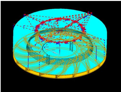
**Fig. 9 Generation of tool path Step for shroud**
