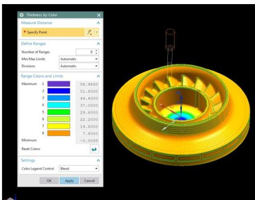
**Fig. 14** shows the tool path generation required for semi-finishing operation.
