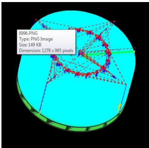
**Fig. 14** Tool path generation for semi-finishing.
