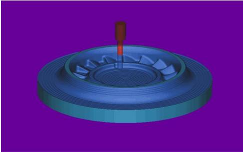
**Fig. 12** Verifying the material removal in 2D dynamics
