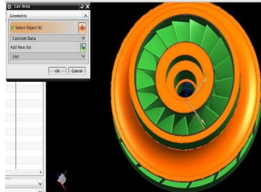
**Fig. 6 Selection of cut area with surface and boundaries curves**
