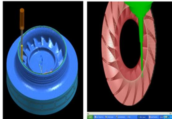
**Fig. 11 verifying the material removal of shroud and vanes in 3D dynamics**
