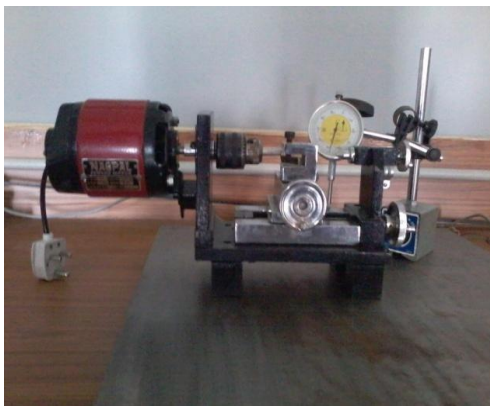
Fig 4 Alignment test on Machine bed
