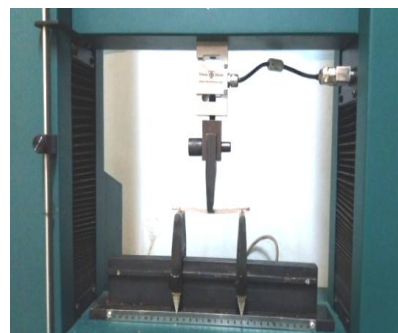
Figure 3 Photographic image of UTM-flexural setup
