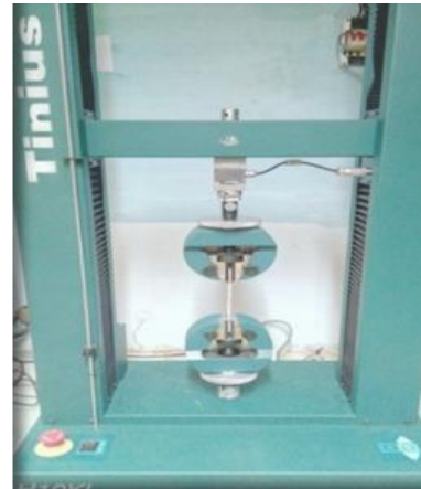
Figure 2 Photographic image of UTM-tensile setup
