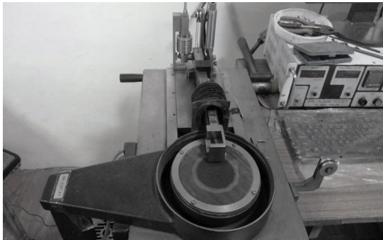
Figure 4. Photographic image of pin on disc set up.
