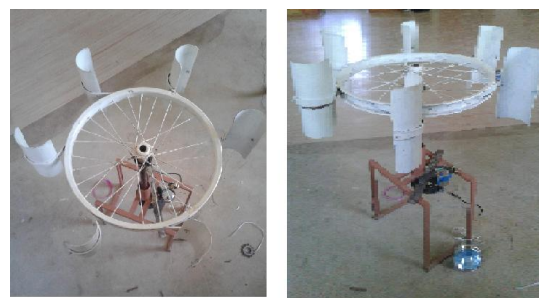
Figure 3 Construction of VAWT
