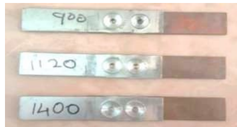
Fig. 4 Single spot-welded pieces at the speeds of 900, 1120 and 1400 rpm
