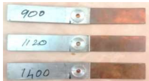
Fig. 5 Double spot-welded pieces at the speeds of 900, 1120 and 1400 rpm
