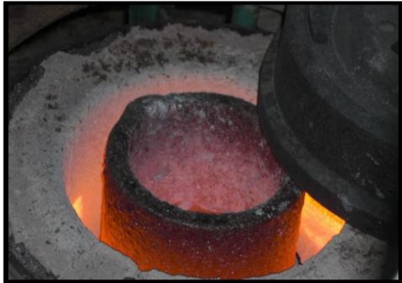
Fig. 2 Al-Si alloy specimen in the crucible.
