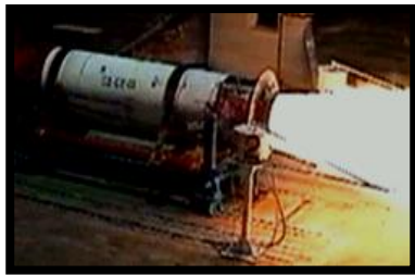
Fig. 2 Ground firing test of rocket motor with flex nozzle system
