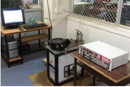
Fig.1. Tribological Test samples and Pin-on-Disc tester
