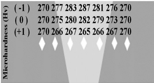
Fig.5 Micro-hardness variation across the interface
