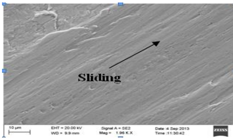
Fig. 4b Worn surface of nitrided SS 316L (N)
