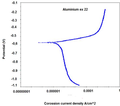
**Fig. 5 Graphical representation of PDP results of a specimen after shot peening Process with optimal value.**
