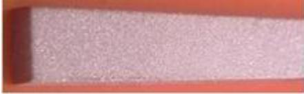
Fig. 2 Photograph of specimen after Shot Peening Process
