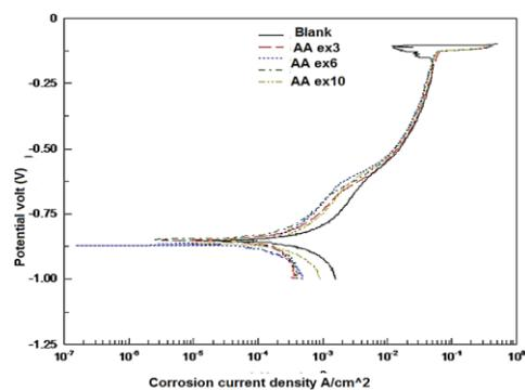
Fig. 4 Cyclic Polarization Curves of Different Specimens
