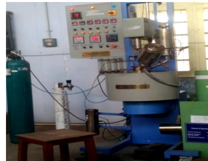
Fig. 1 Squeeze Casting set up
