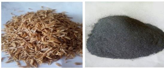
Fig. 1 Showing the reinforcement Rice Husk and Ash. (a) Rice Husk as received condition. (b) Rice Husk Ash in granulated form after Heat treatment (Preheating)
