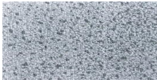
Fig. 1 Microstructure of Mild Steel (MS) 200X
