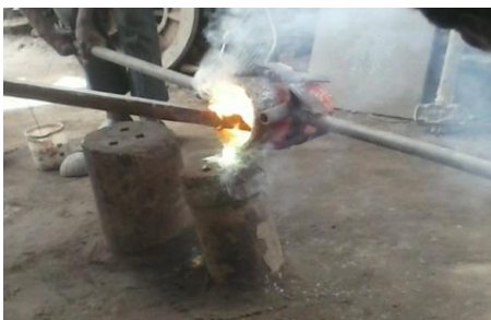
Fig.2 Brass 247/SiC molten metal poured to mould.
