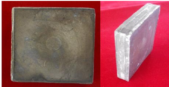
Fig.1 The AZ91/SiC p accumulated diffusion bonding specimen
