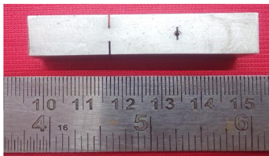
Fig.2.1 Schematic drawing of Shear test specimen
