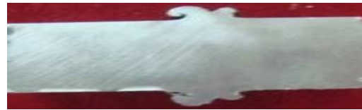
Fig. 5 Cross sectional view of a friction welded sample
