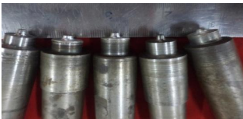
Fig.4 Fabricated FSW tools
