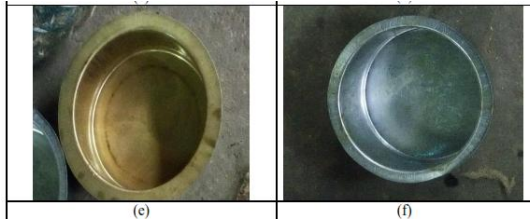
Fig.3. Circular blanks and cups drawn using Hydraulic press. (a) Blank cutting operation (b) Circular blanks use for making cups (c) Hydraulic press use for deep drawing operation (d) Closer view of dies use for deep drawing operation (e) Circular cups made up of Brass and GI (f) Circular cup made up of GI.
