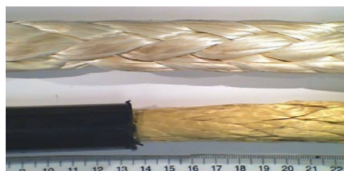
Fig. 2 Handling rope - HMPE (upper), Coated aramid fiber (lower)
