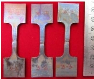
d. Hot tensile specimens after test
