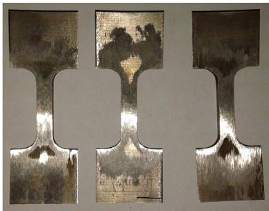
b. Hot tensile specimens before test
