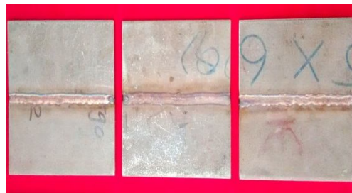
Fig. 2.2 Fabricated Weld Samples
