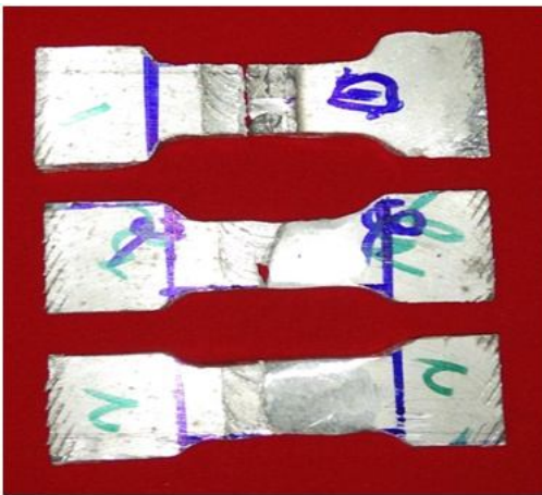
Fig. 3.1 Tensile Test Specimens after Test
