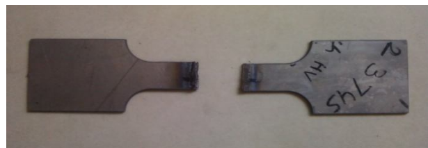
Fig 3. Titanium (Grade 2) and stainless steel (202) GTAW welded plates after tensile testing
