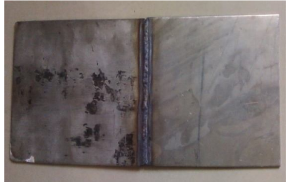
Fig 1. GTAW Welded titanium (Grade 2) and stainless steel (202) plates
