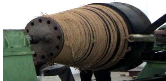
Fig. 1 Tape winding of Divergent Liner
