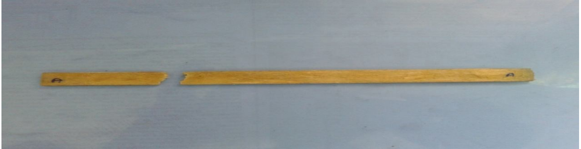
Fig.3 (a) 10% weight composition of 10mm length fiber
