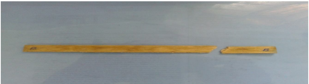
Fig.3 (b) 20% weight composition of 10mm length fiber
