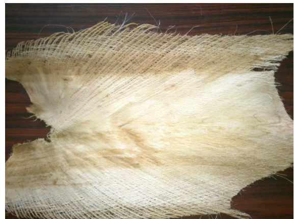
Fig. 1 Naturally woven coconut sheath
