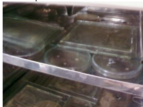
Fig 3.5. Placing moulds inside an oven
