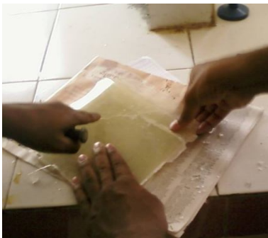
Fig 3.12. Removing the mould
