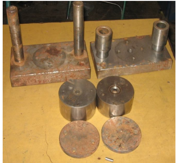
Fig. 3 Tool and die set used in the project
