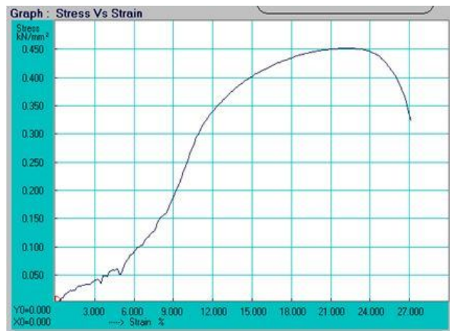
Fig. 8 Tensile test result for SMAW
