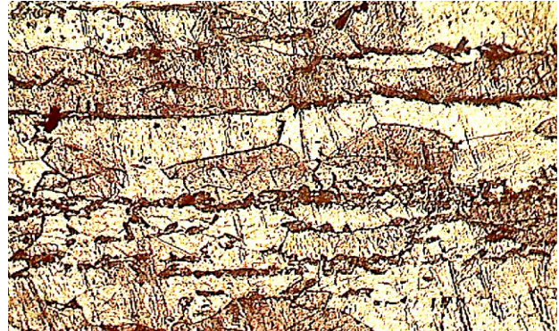
Fig.11(f). Microstructure of 430
