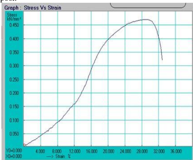
Fig. 6 Tensile test result for GTAW
