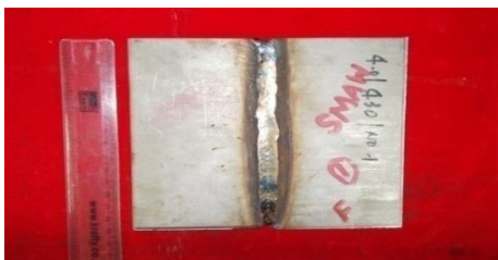
Fig. 1 Welded sample by SMAW
