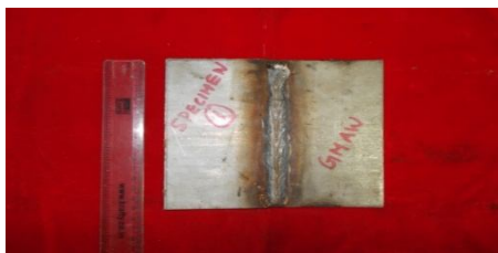
Fig. 2 Welded sample by GMAW
