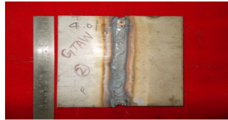
Fig. 3 Welded sample by GTAW
