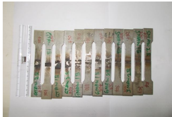
Fig. 4 Tensile samples from the welded plates
