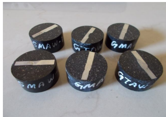
Fig. 5 Microstructure samples from welded plates
