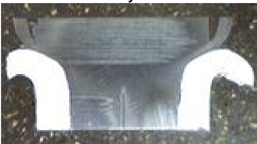
Fig 7. Macro graph of Ti and 304 SS
