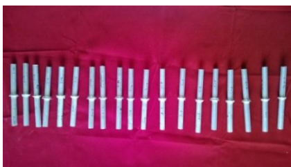
Fig.2 Set of Weld joints
