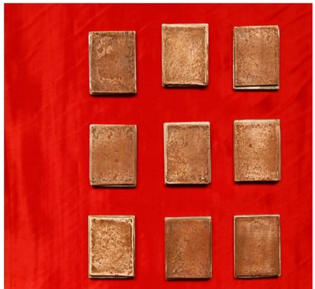
Fig. 3 some of the fabricated diffusion bonds
