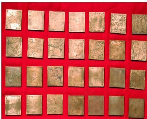
Fig. 1(a) P/M Pure Copper plates
