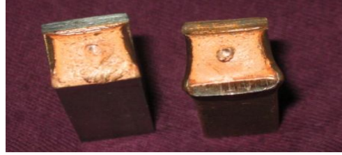
Fig. 5 Fractured sample 3 after impact testing
