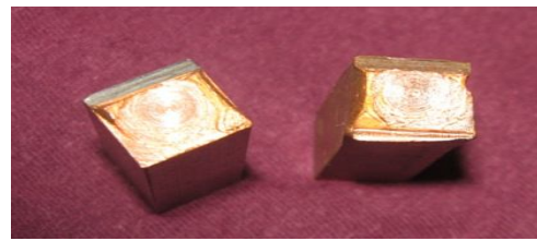
Fig. 7 Fractured sample 5 after impact testing
