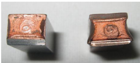
Fig. 4 Fractured sample 2 after impact testing
