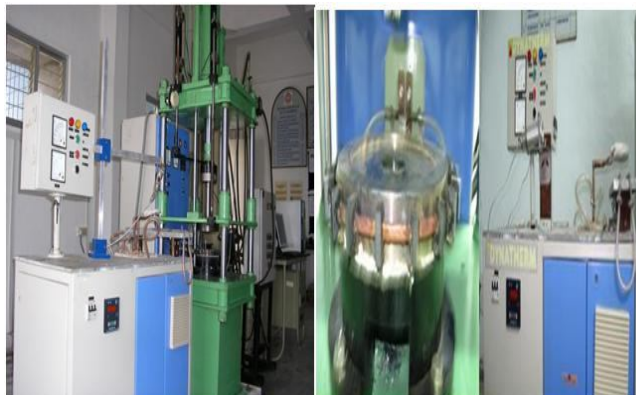
Fig. 1 Experimental Test Rig with Induction Furnace Developed to Draw the High Strength Materials at Elevated Temperature
