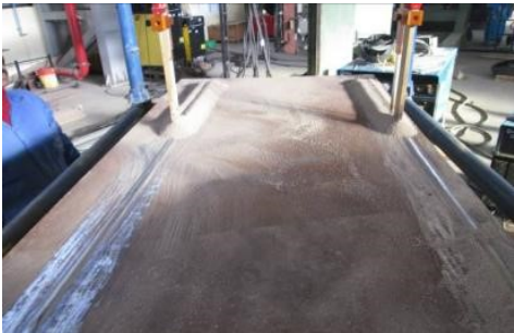
(d) Photograph taken during bead deposition
