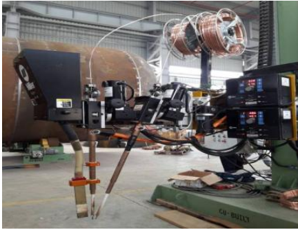
(b) Photograph of solid filler wires with wire feed motors, flux feeder set up
