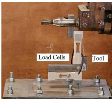
Fig. 2 Pictorial View of a Wear Test Set-up
