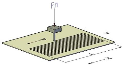
Fig. 1 Schematic drawing of a Wear Test set-up
