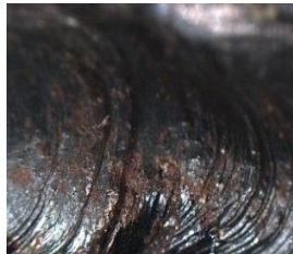
Fig. 5 Image of Insufficient Weld
