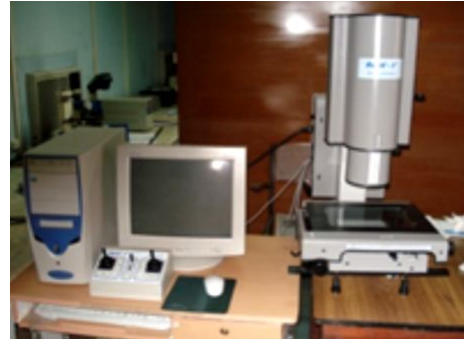
Fig. 1 RAPID I Computer vision system used to capture surface of MIG welding joints.
