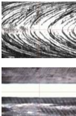
Fig.3 a) Image of Good weld b) Image of no weld
