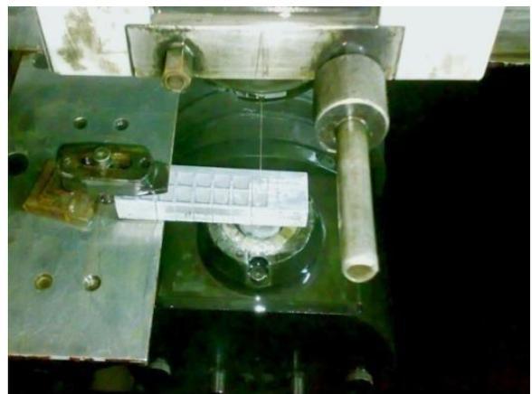
Fig. 1 WEDM of Workpiece
