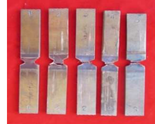
h) Photograph of notched specimen- After test
