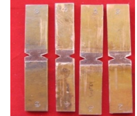
f) Photograph of notched specimen-Before test
