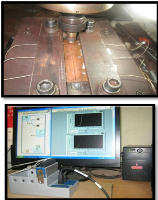
Fig. 3 Temperature measurement using LABVIEW
