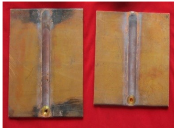
a) Photographs of fabricated joints
