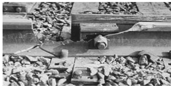
Fig. 7 Fracture in Rail due to Bolt-Hole Crack
