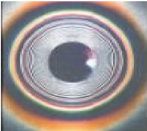
Fig. 2: Photo Elastic Residual Strain Pattern
