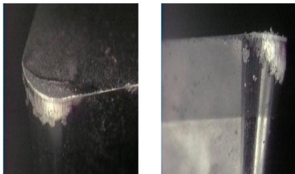
Fig. 7 SEM view of PCD insert after 10 min turning
