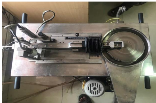
Fig. 2 Pin on Disc Apparatus
