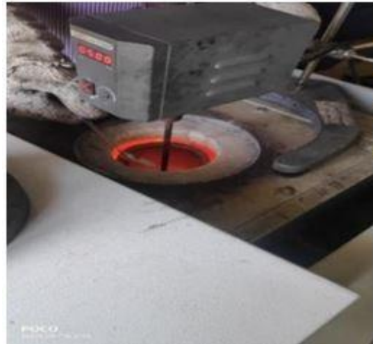
Fig. 1 Stir Casting Process
